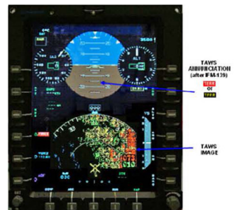
TAWS displayed as HSI underlay on PFD
