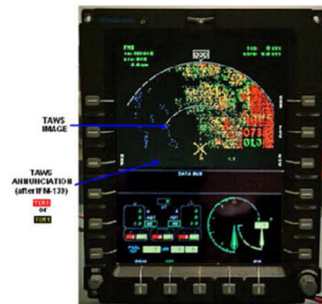
TAWS displayed on MFD Map/Radar page
