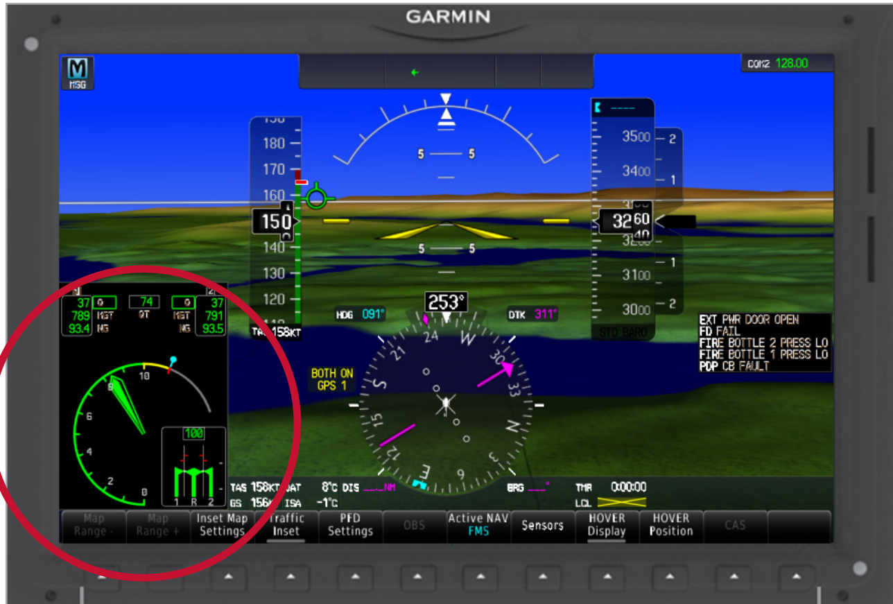
Power Situation Indicator (PSI).
